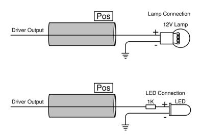
**Note:** The connection to the Mercury ECU changes with the GP Output Priority selection, View the Priority spreadsheet for the specific firmware to see which output is selected. Then make sure on how to connect between the 2 options above. It could be connected on a negative or positive driver.
